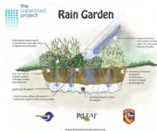
Typical Rain Garden Source: www.thewatershedproject.com
